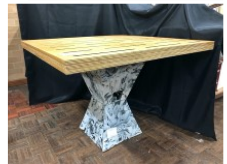
Angus McLean was able to create an innovative picnic table that was able to harvest and store rainwater. The fact that the base was made entirely from recycled milk containers added to the environmental credentials of the project.
